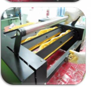
Step 3: The handle is swinged forward to cut the excessive dough and sharp the curry puff
