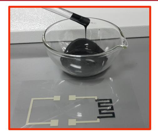
The innovation is composition of materials and preparation method in producing thick film paste for screen printing, composed of organic binder using linseed oil mixed with certain active powder.
